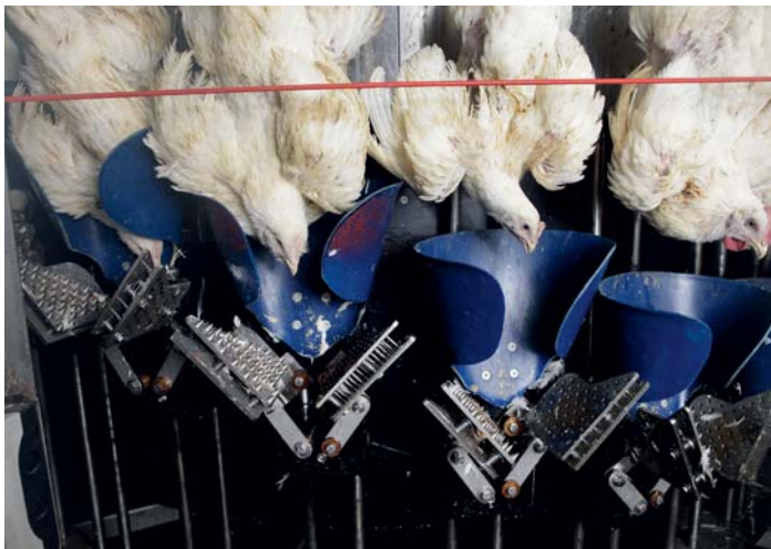
The birds are smoothly captured into a cone, which is made of flexible polyurethane and which is closing proportionally.
